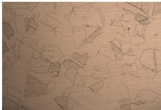
Fig. 1 Optical micrography of STS 304L stainless steel (x200)
