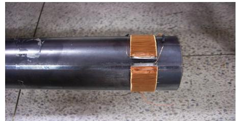
Fig. 4 Toroidal coil wound around the nickel strip attached to the pipe
