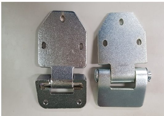
(a) Cr/Zn coating specimens
