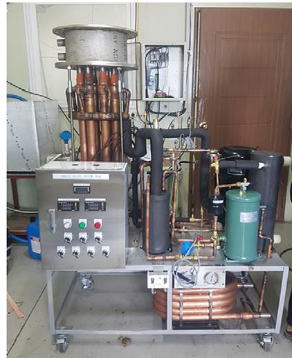
Fig. 1 Experimental equipment of the seawater cooling system
