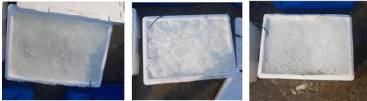
(a) Slurry ice (b) Crushed ice (c) Chilled water
