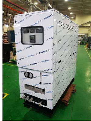
Fig. 4 Photographic of sea water slurry ice maker
