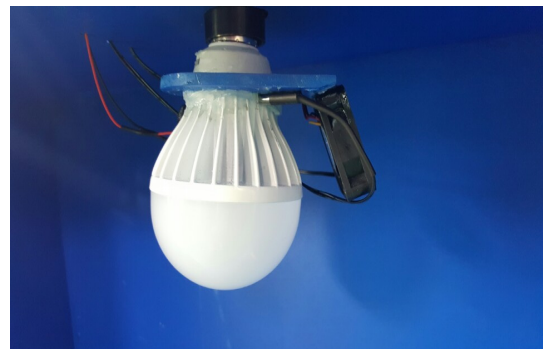
Fig. 5 Systematic diagram for the attachment of convection fan and temperature sensor
