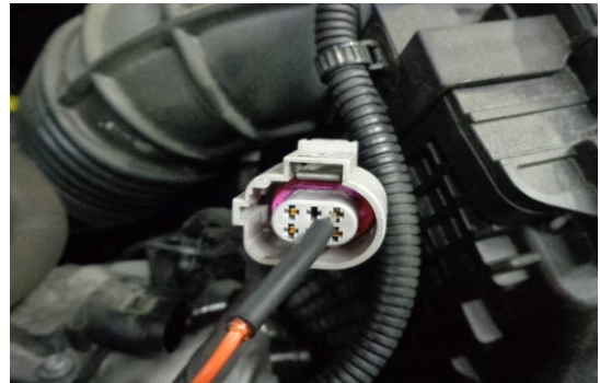
Fig. 13 Check the pin tension
