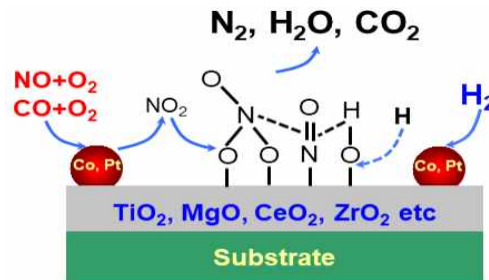
Fig. 5 Mechanism of simultaneous harmful gas reduction of H 2 -SCR
