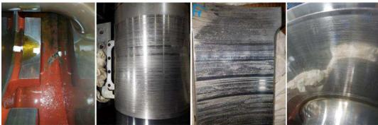
Fig. 6 Overhaul Inspection for thrust bearing
