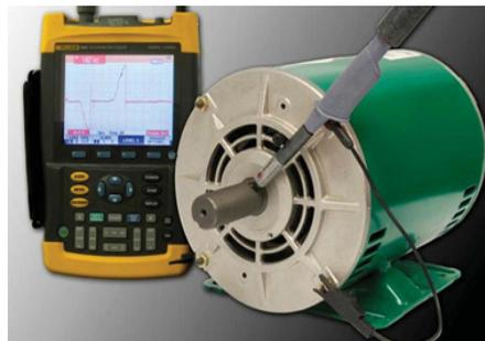
Fig. 10 Equipment for shaft voltage measurement
