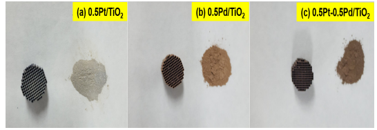
Fig. 2 Image of catalyst powder and coated catalyst after calcination of H 2 -SCR
