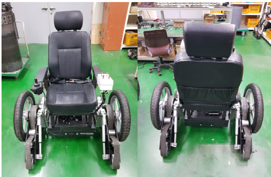
Fig. 10 Electric wheel for moving stairs
