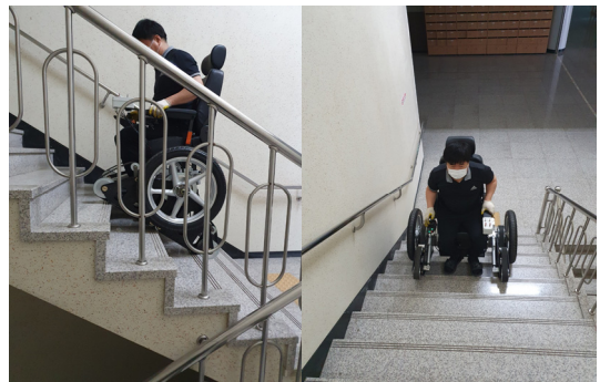
Fig. 13 Photo of electric wheel when moving stairs
