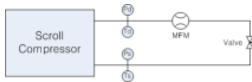
Fig. 1 Schematic diagram of simple scroll compressor test setup
