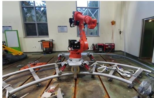
Fig. 7 Prototype of the mobile manipulation system for pier construction
