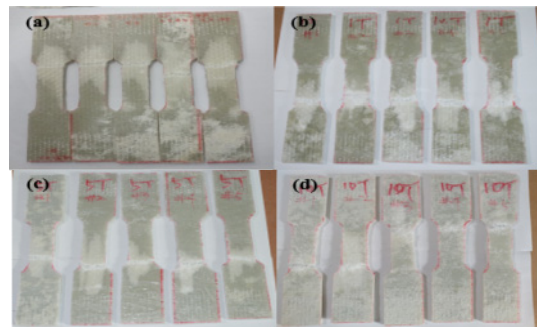
Fig. 9 Failure patterns (a) neat resin, (b) AL5L-1, (c) AL5L-5 and (d) AL5L-10 of tensile test
