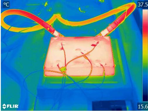
Fig. 5 Battery temperature distribution of single cell at the end of discharge taken by the thermal imaging camera
